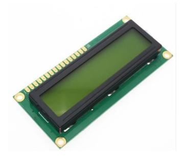
The **1602** stands for 16x2 which is 16 characters wide and 2 lines tall. The default board has 16 pins which is a lot to hook up. Fortunately, there is a corresponding controller, the **HD44780**, that goes with it.
